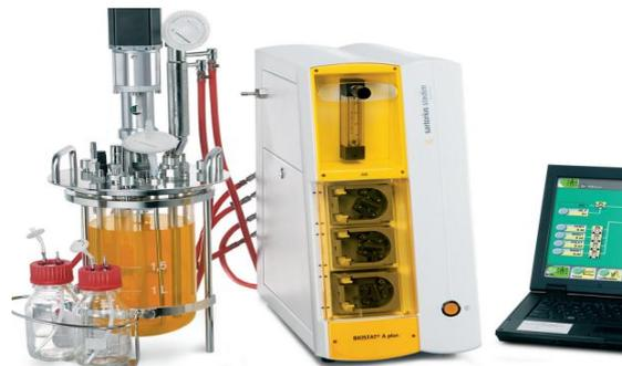
**Figura 7** Partes del biorreactor BIOSTAT® “Culture Vessels and Equipment UniVessels®”<sup>77</sup>
